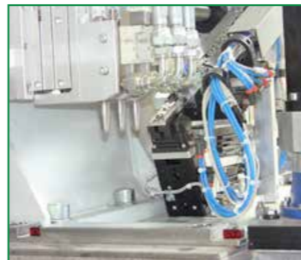
Inserimento colla e basetta Glue and hinge-plate insertion
